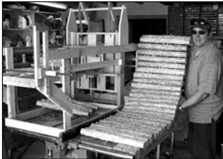
YIP team member Bruce Harshman displays a straw cable mat, created by the prototype loom.
