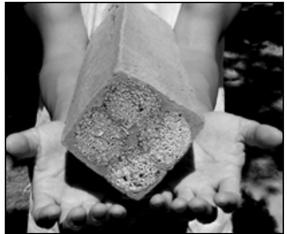
TOP: Field testing of the Strawjet Harvester in Fall '05. BOTTOM: A treated Strawcore member.
